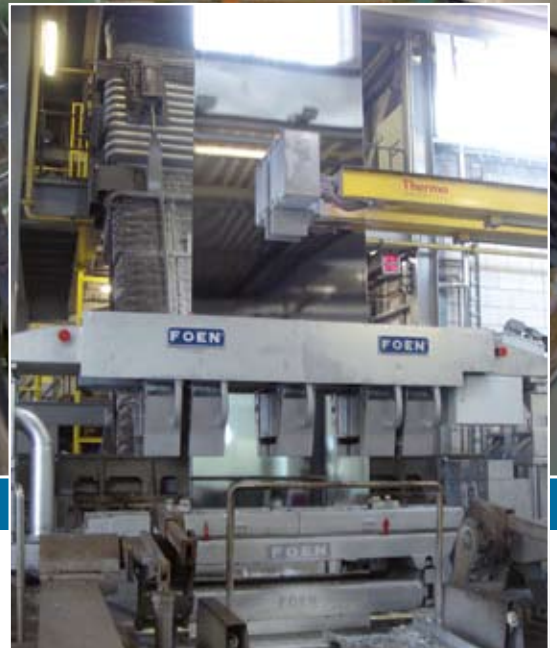
Non-contact electromagnetic strip stabilization for galvanizing lines
